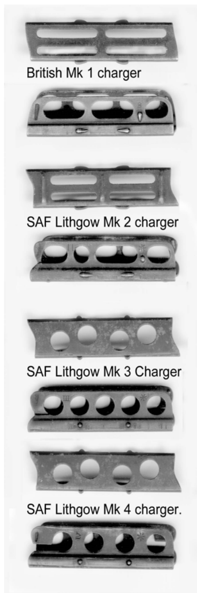
FIGURE 4. English Mark I and SAF Lithgow made Mark II,III and IV .303 Chargers
