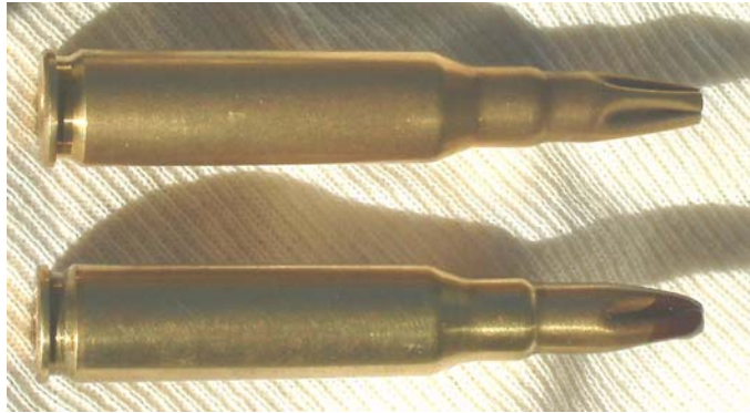
FIGURE 9. Full length brass blanks : top Footscray F8 , bottom English L10A2
