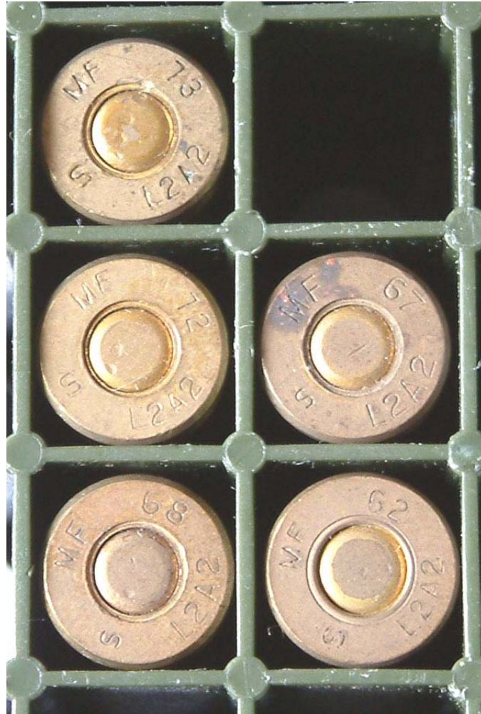
FIGURE 4. Examples of 7.62 Ballistic Standard cartridges from 1962 -1973, Note the 'yellow' primer lacquer which is a requirement of 'standard' ammunition
