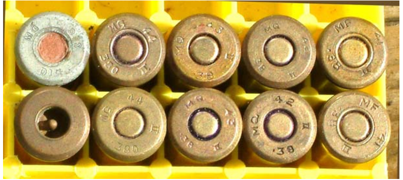
FIGURE 1. Local .380 ammunition : from the right No1 Factory 1941 production, Rocklea 1942 & 1943 production and No2 Factory 1944 production. At top left is an undated tinned drill D Mark 1* made by the No2 factory and at bottom left an unmarked 'drill' reported as being made at Rocklea.
