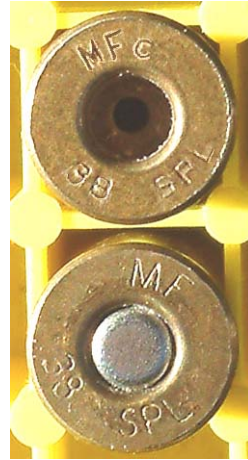
FIGURE 6. .38 Special revolver cases : the top example carrying MFC (Commercial) identification the lower carrying MF only.
