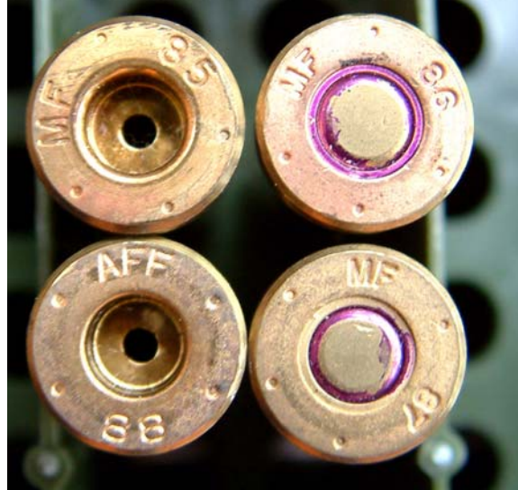
FIGURE 5. Gulf and Western Plant made 7.62 cases 1985-1988: Note the boxer primer configuration and the change of headstamp to AFF in 1988.
