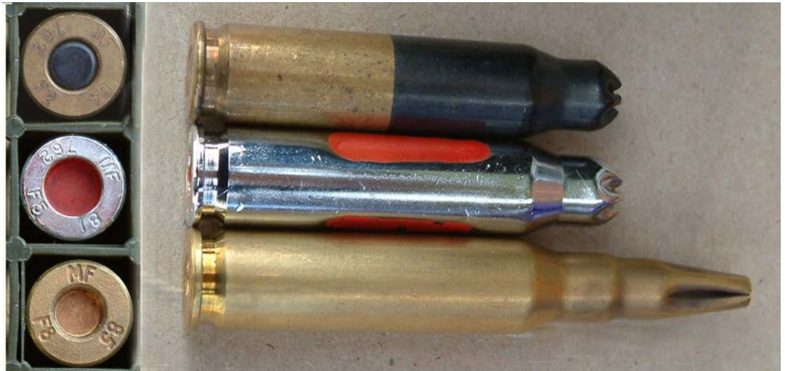
FIGURE 6. Inert non-bulleted 7.62 : from top a black primer inert F2 grenade launching blank, a F5 Drill Grenade Launching Cartridge and an inert F8 blank
