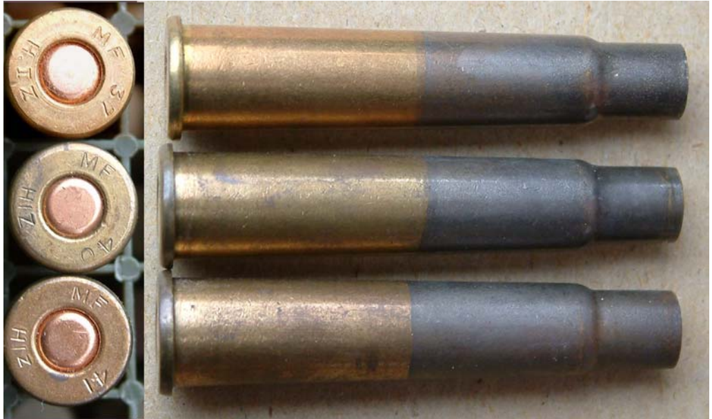
FIGURE 2. Some typical HIZ Rifle Grenade Cartridges made by the No1 Factory showing 1937, 1940 and 1941 specimens.
