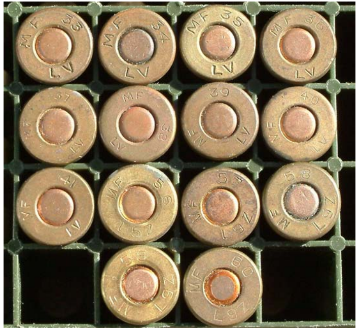
FIGURE 6. This figure shows the headstamps of Footscray made L mark V blanks 1933 - 1956 and L mark 9 types made from 1957 to 1960.
