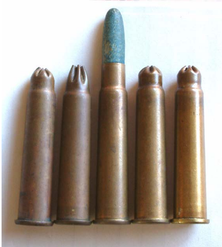
FIGURE 2. From left to right : Early CAC .303 blanks with short and long mouth crimp in unheadstamped cases, a 1944 Footscray wood bulleted blank, the last of the Mark 5 blanks of 1956 and the Mark 9 type 1957-1960.
