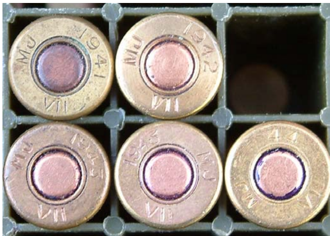
FIGURE 4. .303 ball headstamps of the No4 SAAF Hendon 'MJ' 1941-1944.
