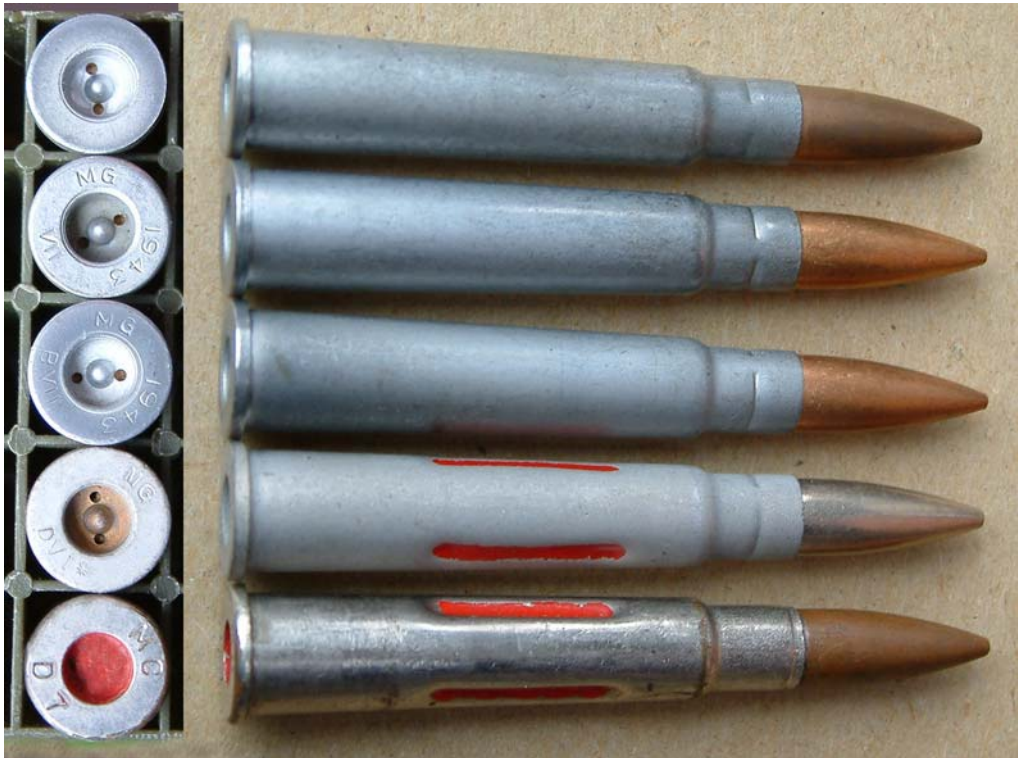
FIGURE 5. No 2 Factory drills and dummies: From top : Unheadstamped Mk V inspection dummy, two more Mk V Inspector dummies made from surplus ball and Incendiary cases respectively, A Mark VI* fluted drill circa 1944 and a Chromium plated Mk 7 drill circa 1948.
