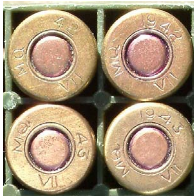
FIGURE 7. .303 ball headstamps of SAAF Nos 6&7 Rocklea 'MQ' 1942-1943
