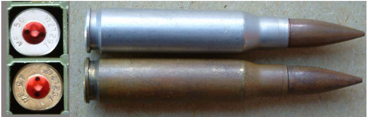
FIGURE 1. Early inert 7.62 cartridges : Top a 1956 tinned dummy made from L2A1 case, Bottom : a 1957 inert round made from a L2A2 case.
