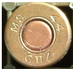
FIGURE 2. A Mark GIIZ tracer marked ‘MS’ loaded at the Explosives and filling factory at Salisbury.
