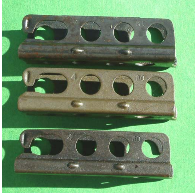
FIGURE 1. .303 Chargers: At the top a Mk IV made by MO ( Maribyrnong Ordnance), with a drab olive and conventional black phosphated Mk 4 made at BO ( Bendigo Ordnance)
