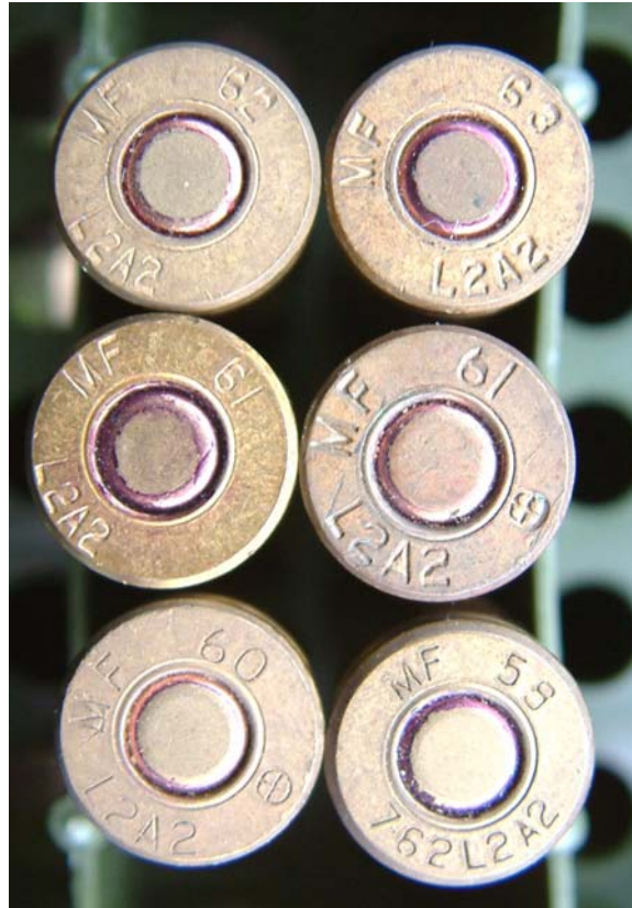
FIGURE 1. 7.62 Ball round headstamps 1959 through 1963 showing introduction then deletion of the NATO symbol .
