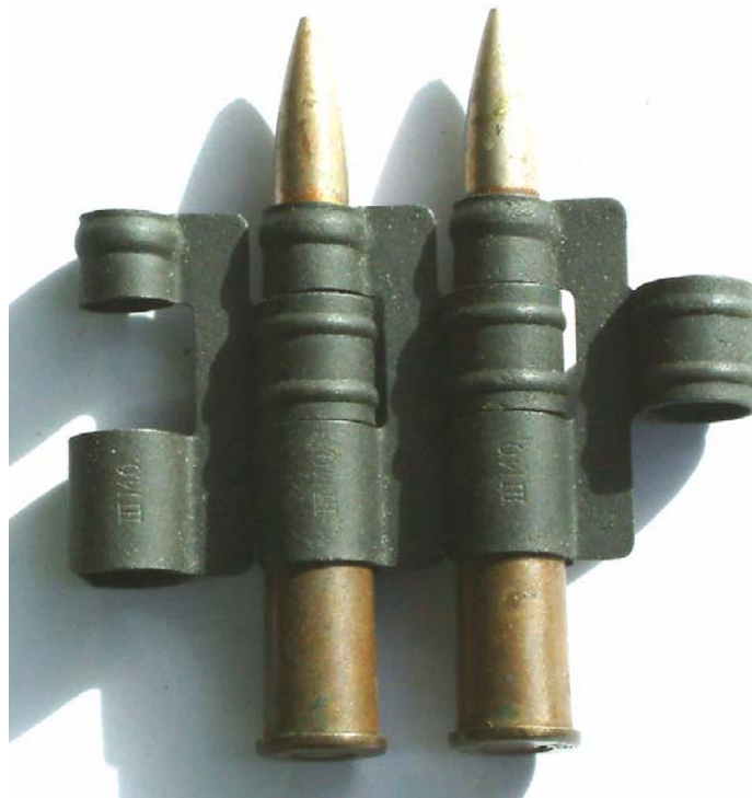
FIGURE 2. An example of Vickers link belt showing Mk III links which were made at OFM.
