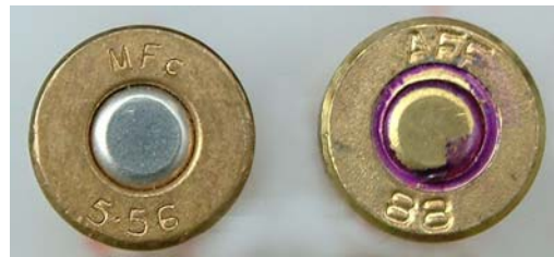
FIGURE 9. Commercial .223 W ( 5.56 ) of the 70's headstamped MFC compared to Military 5.56 of 1988
