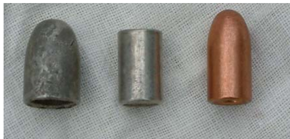
FIGURE 5. Some commercial handgun projectiles : from left .45 tinned lead projectile, .38 tinned lead wad cutter and jacketed .38 projectile.
