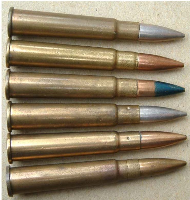
FIGURE 10. Bullet retention in Tracer , Incendiary and Armour Piercing cartridges : from top cupronickel and gilding metal tracers with press fit and mouth coning, Blue tipped incendiary with press fit, cupronickel and gilding metal AP rounds with punch neck staking (prior to 1942) and AP with full neck staking
