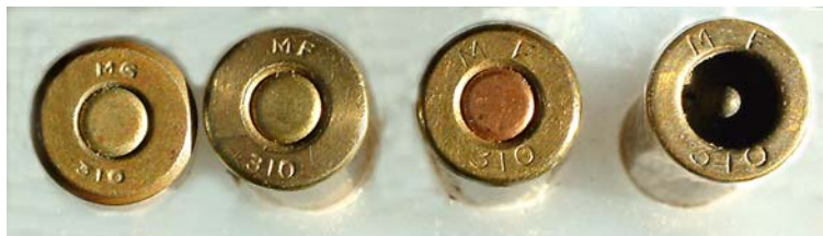
FIGURE 6. Headstamps of Footscray .310 Cadet cartridges. From right an unprimed 1929 cartridge featuring provision for the .455 primer, A 1930's specimen with small copper primer and WW2 No1 and No2 Factory specimens with brass primers.
