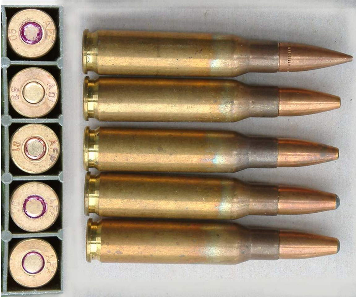
FIGURE 11. Non-military 7.62 loads of the early 1990's from top 1990 full metal jacket 170 grain boat tail bullet, 1993 and 1991 hollow points, a 1991 soft point and an undated soft point.
