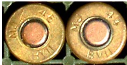
FIGURE 7. Example Headstamps for 1944 and 1945 Hendon incendiary production.
