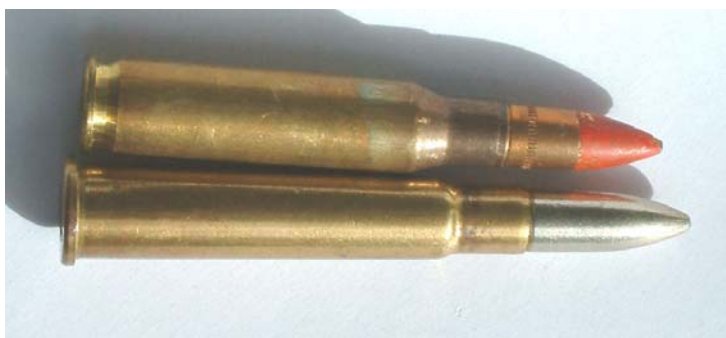
FIGURE 3. The Footscray made F3 tracer with blunt ogive shown against similar shaped .303 English G8 tracer .
