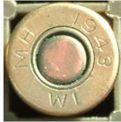
FIGURE 2. An example of Hendon 1943 .303AP production headstamp.
