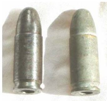
FIGURE 6. 9mm Inspection rounds U Mark I: from right 1960 tin coated solid brass, 1955 all steel.
