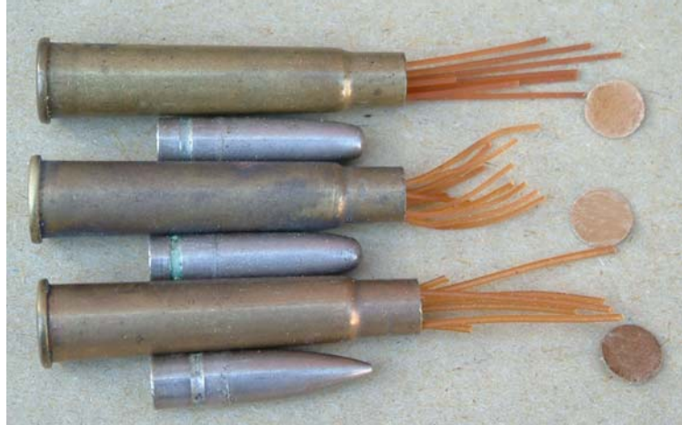
FIGURE 7. The components of MK II, VI and VII rounds. From top the Mark II with cordite size 3 3/4 (usually about 60 strands) , centre the Mark VI also with cordite size 3 3/4 and lower Mk VII with the ‘thicker’ cordite MDT size 5/2 (usually 36-40 strands ). Note the glazeboard wads and that the Mk II and Mk VI projectiles are not externally different.
