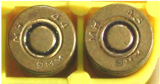
FIGURE 4. Hendon 9mm headstamps for 1943 and 1944 production
