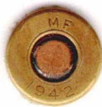
FIGURE 4. An early No1 plant (MF) incendiary round. A similar format MG 1942 and MH 1942 incendiary rounds are reported
