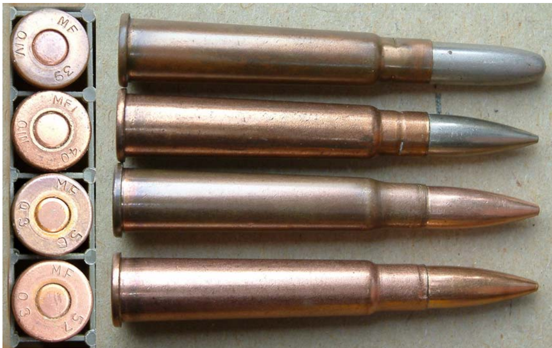
FIGURE 6. Some .303 proof specimens : From top a Mark IV of 1939 manufacture, a mark III from 1940 and Mark 3's from 1956 and 1957.
