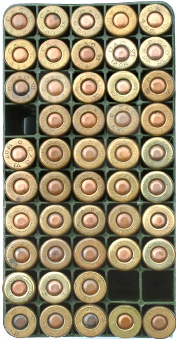
FIGURE 1. CAC Cartridge examples of early .303 Mk II and undated Mk VI (lower 2 rows) and month year dated examples from May 1906 to March 1909 ( row 3 from bottom to top).
