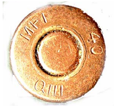
FIGURE 1. An example of the MF1 headstamp used in early 1940 for a short period. The item shown is a .303 proof Mk III round
