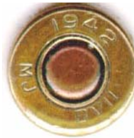
FIGURE 6. An example of MJ 1942 BVII incendiary round headstamp. These rounds carried blue tip markings and blue primer lacquer
