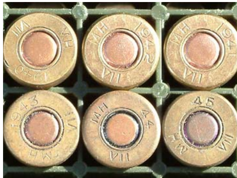
FIGURE 3. .303 ball headstamps of No 3 SAAF Hendon 'MH' 1940 -1945
