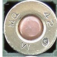
FIGURE 2. A Ballistic Standard .455 Webley Round made at Rocklea.
