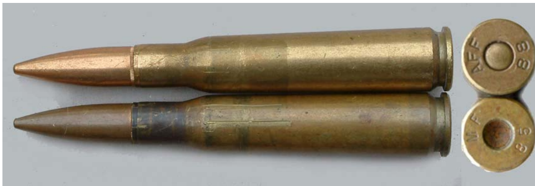
FIGURE 3. Top a 1988 50 Browning specimen headstamped with the AFF identifier and below an inert specimen with blind primer pocket dated 1985 and used at Ordnance Factory Bendigo during setting up the M9 link programme/
