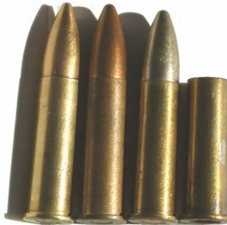
FIGURE 7. A side view of the cases shown in previous figure. Note the Nickel projectile from 1930's production and gilding metal projectiles in the WW2 production items
