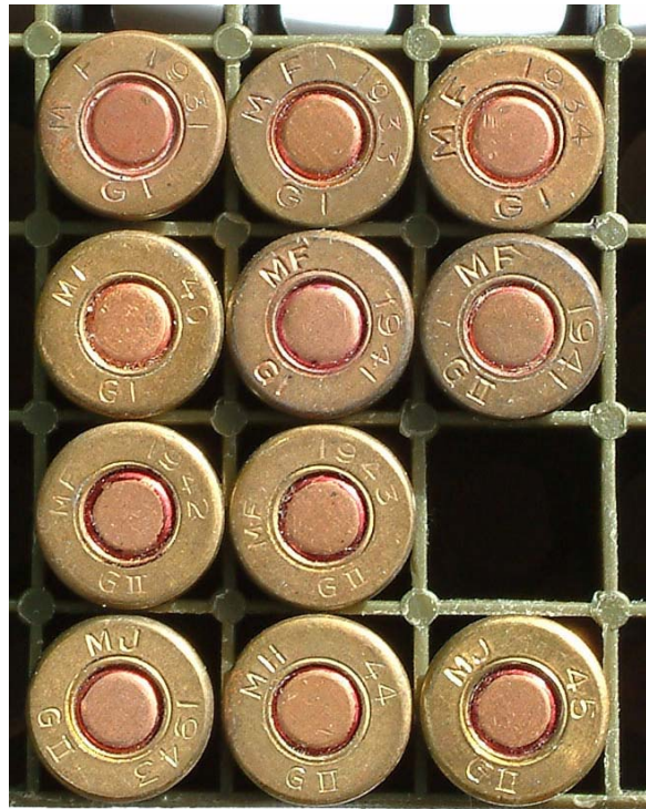
FIGURE 1. Examples of Footscray and Hendon Tracer Headstamps showing early 30's examples and the change from G1 to GII marks in 1941.
