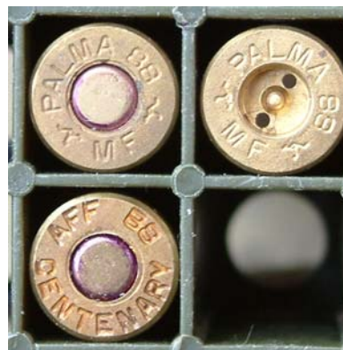
FIGURE 9. Headstamps of the Centenary and Palma Match 7.62 rounds also showing Berdan priming.
