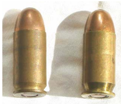
FIGURE 13. .45 Auto cartridges : right a typical WW2 No2 Factory round with case cannelure and a 50's 'MF' round without case cannelure.
