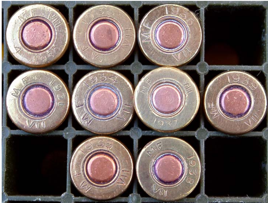
FIGURE 6. Headstamps of Footscray made Air Service .303 ammunition from 1930 -1939. Note variations in layout and format in the 1930 and 1937 specimens
