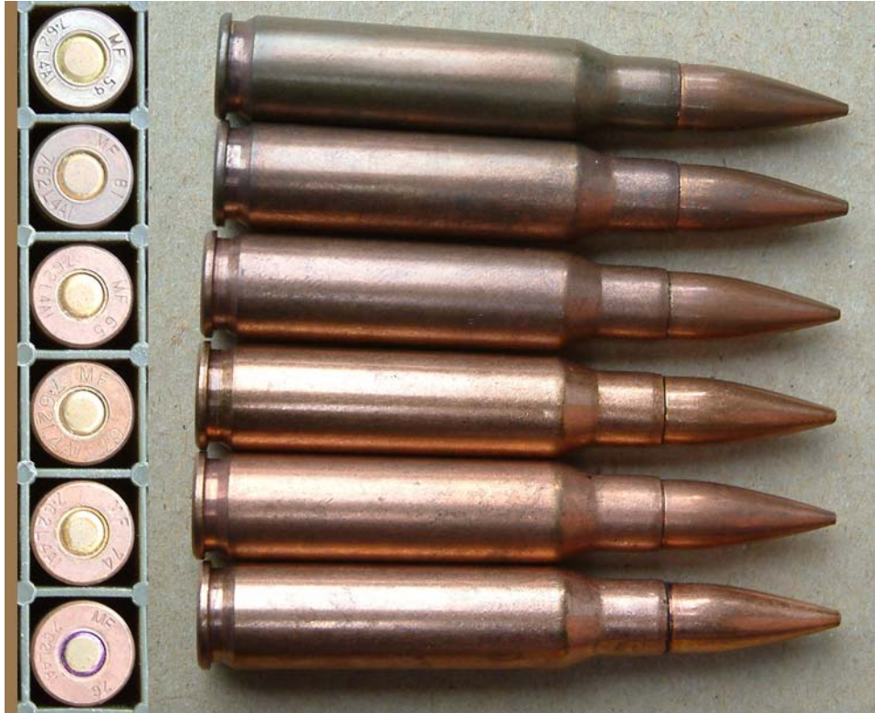
FIGURE 7. Some copper washed 7.62 L4A1 Proof rounds : from top 1959, 1961,1965,1972, 1974 and 1976 specimens
