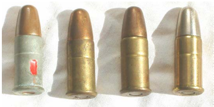
FIGURE 2. Local .380 ammunition; From right a cupronickel jacketed specimen from the No1 factory (1941), a Rocklea specimen (1942,43), a No2 factory specimen (1944) and a tinned, undated fluted drill from the No2 factory (circa 1944).
