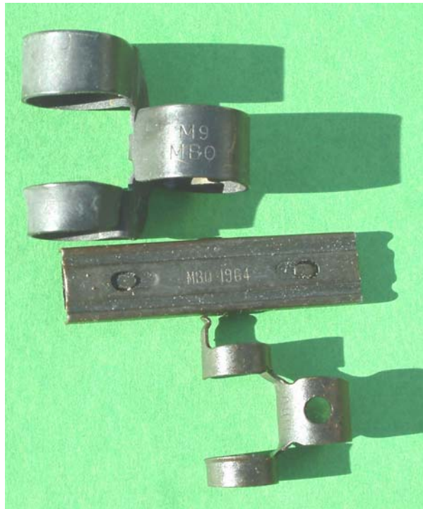
FIGURE 2. From top : 50 Browning M9 link circa 1980's , 7.62 charger made in 1964 and the 7.62 M13 link for the M60 machine gun made at Ordnance Factory Bendigo and carrying the MBO mark.
