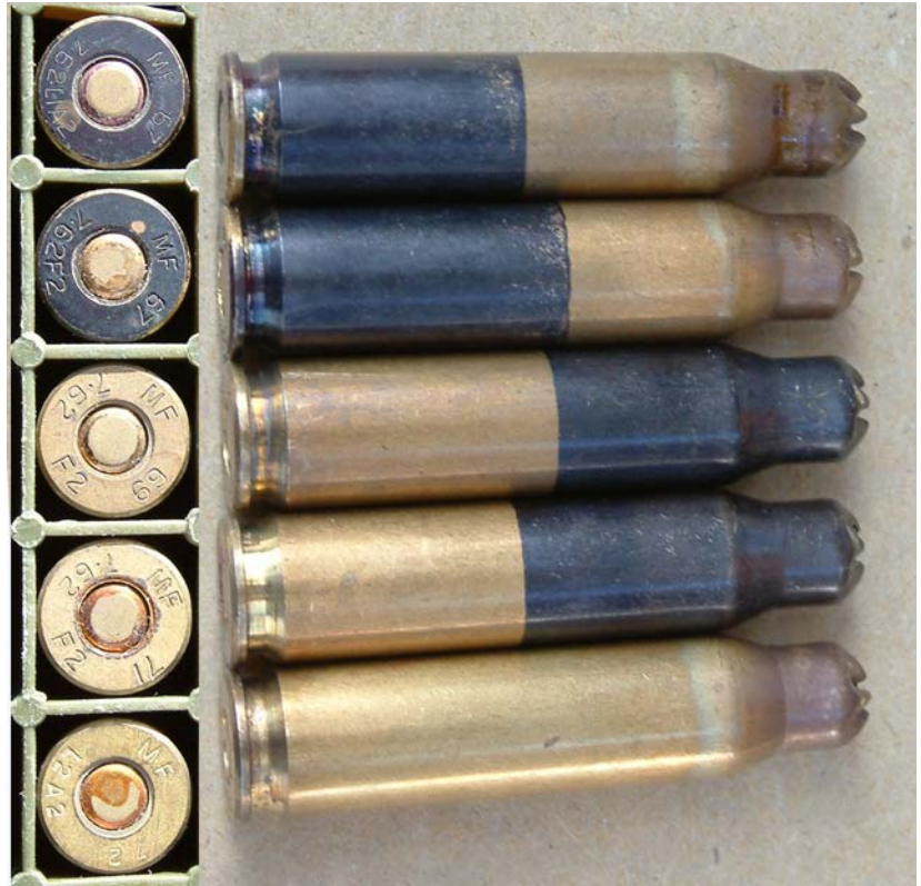
FIGURE 2. Grenade cartridges : from top a 1967 L1A2 pattern, a 1967 F2 pattern then 1969 and 1971 F2 specimens and finally an unknown variant using un-blackened 1972 L2A2 ball cases. Note that the first 1967 F2 cartridges had the lower portion of the case blackened but this was changed to upper half blackened in later specimens
