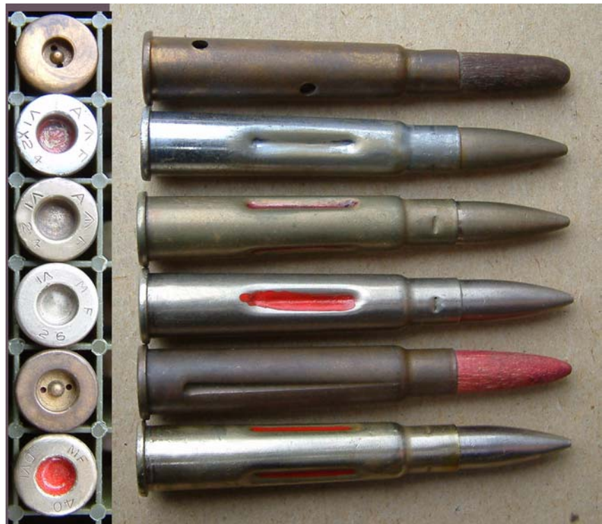
FIGURE 1. .303 Drill Rounds : From top : A typical CAC era (1915) wooden bulleted Mark III drill, A 1924 Chromium plated Mk VI drill, A 1924 white metal Mk VI drill , A 1926 whitmetal Mk VI drill. a WW2 expedient drill Mk VIII and a 1940 whitmetal drill Mk VI
