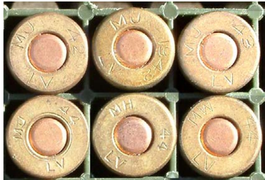
FIGURE 4. Correctly identified L Mark V Blanks made at the WW2 factories Welshpool (MW) and Hendon (MH & MJ) . Many blanks were also made from redirected ball cases
