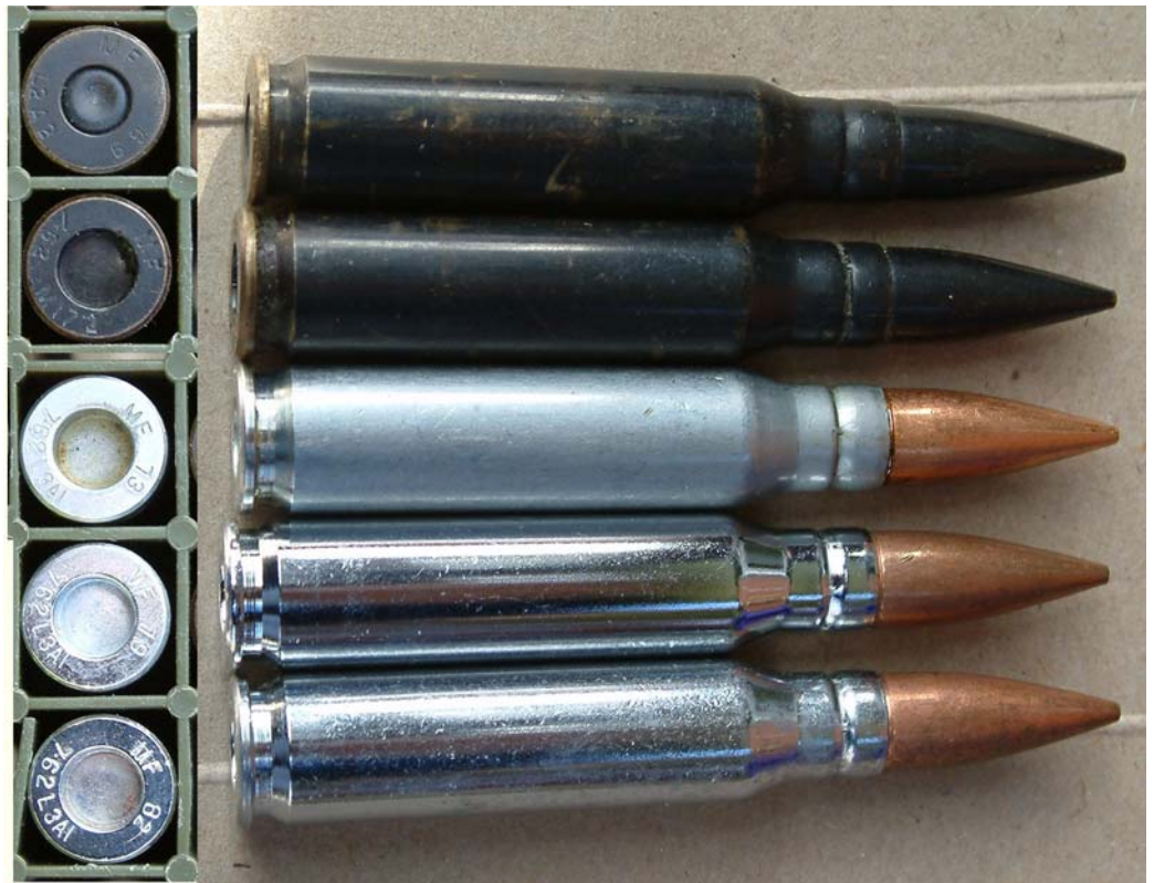
FIGURE 4. 7.62 inert rounds : at top two blackened M172 pattern circa 1969, a whitened L3A1 inspection dummy of 1973 and at bottom two chromium plated L3A1 dummies from 1979 and 1982 respectively.
