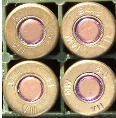
FIGURE 8. .303 ball headstamps of SAAF No 7 Welshpool 'MW' 1942-1945
