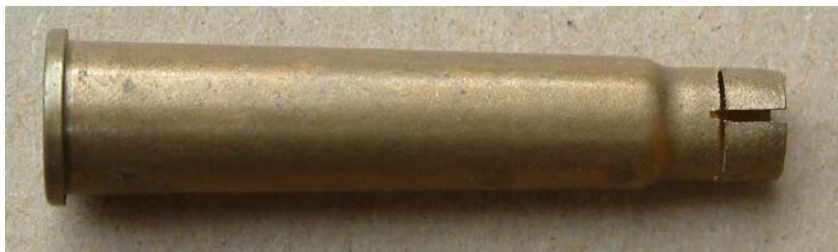
FIGURE 5. A Murray Switch case : Primed ball cases were prepared with specially slit necks to be used in the Switch Combination Aust. Mark 1
