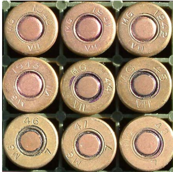
FIGURE 2. .303 ball headstamps of the No2 SAAF Footscray 'MG' from 1940 to 1948
