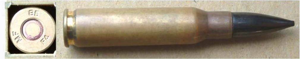
FIGURE 9. A Blackened Projectile inert round made at Footscray in 1984 - purpose unknown
