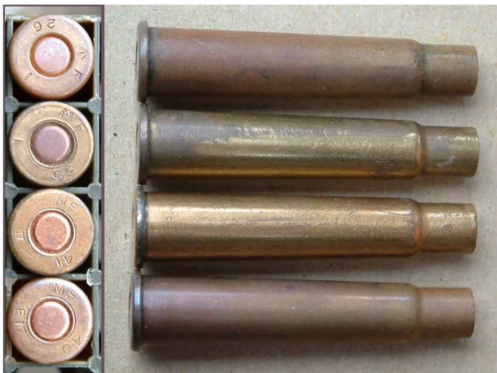
FIGURE 1. Rifle Grenade and other discharger cartridges: from top : 1926 rifle grenade Mk 1, 1935 rifle grenade Mk 1, 1941 unknown type , and 1940 Smoke discharger cartridge EIT.
