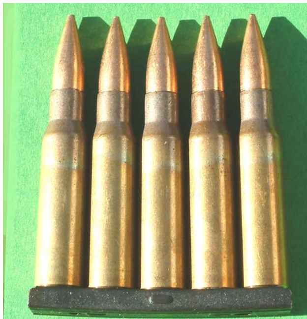
FIGURE 3. The 5 round 7.62 charger with black phosphated steel body and spring steel inner platform made at Ordnance Factory Bendigo from the early 60's.
