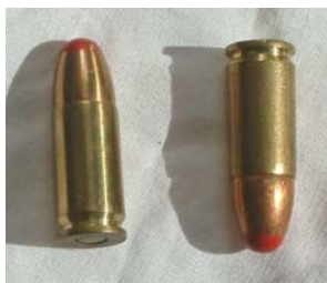
FIGURE 11. Red tipped 9mm rounds made at the No1 Factory in 1943 and reported as being early proof rounds
